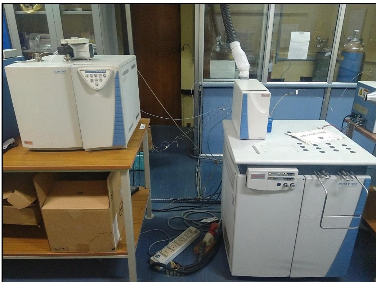
**Figure 2.5:** Photograph of Flash 2000 elemental analyzer interfaced with Delta V IRMS through Conflo IV at GeoSIL, PRL, Ahmedabad, India (Photo Credit: Deepak Kumar Rai).
